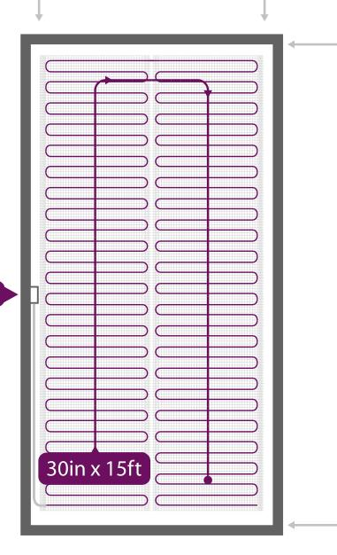
Cut the white mesh to shape the mats to fit any room. Any combination of mat sizes can be used up to 150 square feet per thermostat.
