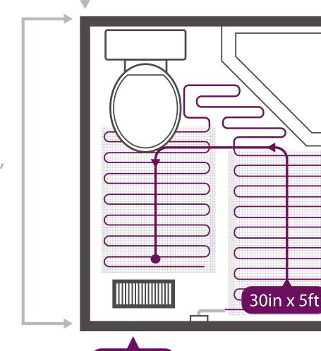
Cut the white mesh to shape the mats to fit any room. Any combination of mat sizes can be used up to 150 square feet per thermostat.
